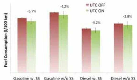
Figure 4: Impact of UTC on emissions of different passenger cars in the city of Turin. SS: stands for start-and-stop system
